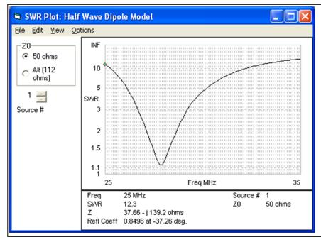
The SWR has gone down and that the bandwidth has been narrowed somewhat. This is because the feed line is contributing to the resonance.
