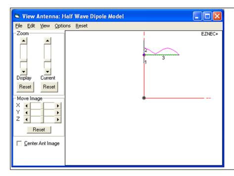
33% off center fed dipole using ¾ wave feed line. The feed line currents are now significant and major changes in antenna performance are expected.
