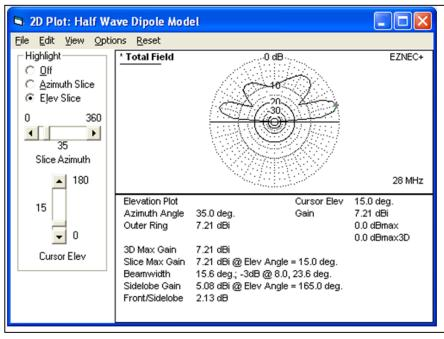
Indeed. The gain pattern is now no longer symmetric and has increased to over 7 dBi. Actually, this antenna now operates more like a horizontal antenna.
