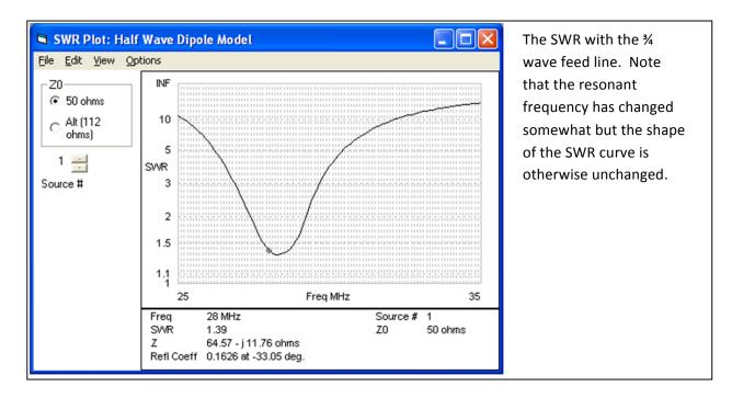
Up to this point, the feed line has had a relatively minor impact on antenna performance. As it turns out, feeding the dipole with a feed line which is perpendicular to the dipole and at the center is the *best* case.
