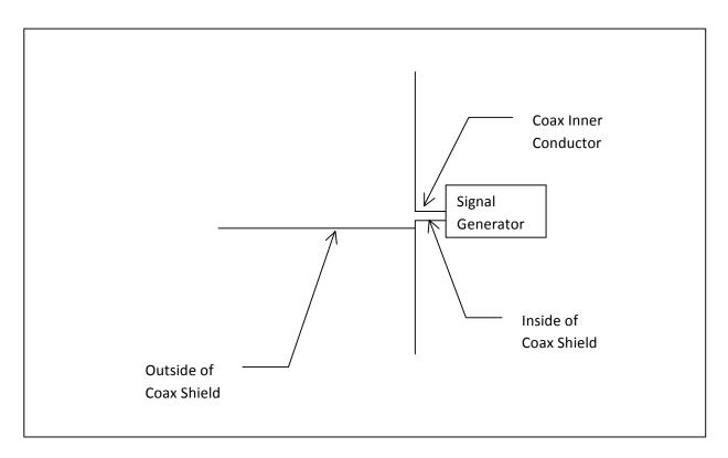
Thus, the coax feed line can be modeled as a single conductor and the signal generator can be placed directly on the dipole.
