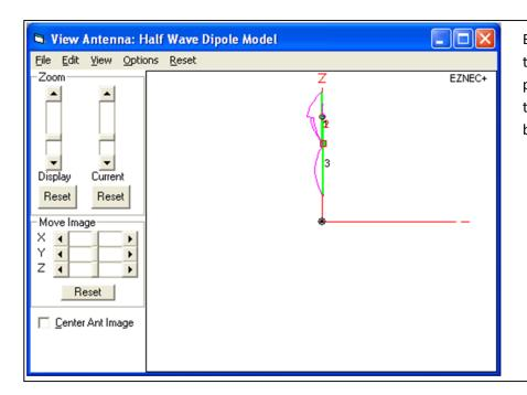
Back to one choke but this time not at the feed point. Rather, it is on the feed line at the bottom of the dipole.
