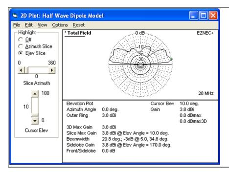
Note that the gain has gone up somewhat and the optimal launch angle is reduced. These are generally accepted as improvements.
