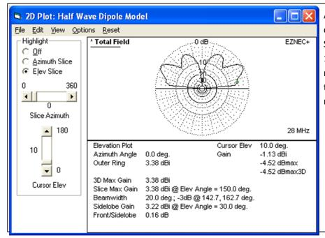
Antenna gain has changed dramatically. Specifically, the gain at 10 degrees has been reduced from 2.72 db in the first simulation to minus 1.13 db here.
