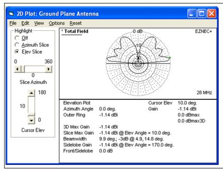
Gain pattern of elevated ground plane antenna with resonant feed line and perfect choke. Max gain, -1.14dBi.
