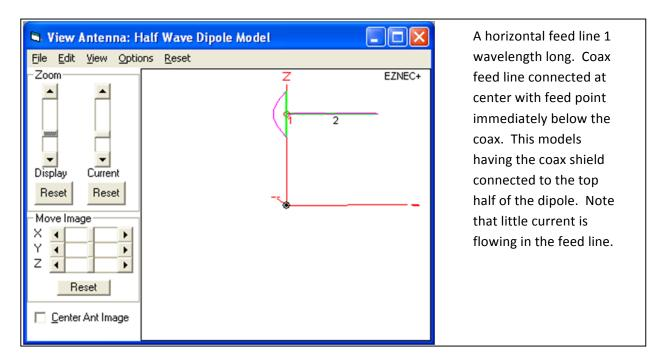
To look more closely an examination of the 'currents' file is in order. Here is a piece of the 'currents' file for the feed line (wire 2 above). Note that there is, in fact, some feed line current but that it is quite small. While wire 1 has peak currents of 1 amp (the specified drive), the feed line has peak currents of only .07 amps.
