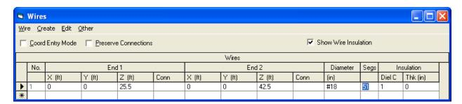
This single wire is the starting point of the exploration of feed line currents. It is a 28 MHz, resonant, vertical dipole antenna placed 1 wavelength above ground.
