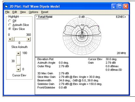
The gain pattern is returned to the original. The feed line now has no effect on the antenna performance.
