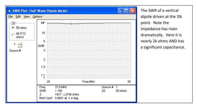
This last point should be emphasized. The drive impedance of a resonant dipole near its endpoint is very high. Consider a simple calculation. Suppose the antenna is expected to carry 5 watts. To drive 5 watts into this antenna will require a voltage of V = sqrt(P\*R) or V = sqrt(5\*2000) = sqrt(10000) = 100 volts. Even higher voltages can occur if the feed is even nearer the endpoint.
