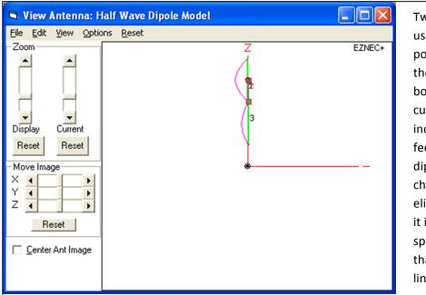
Two perfect chokes are used. One at the feed point. The second is on the feed line level to the bottom of the dipole. If currents are being induced because the feed line is 'close' to the dipole, this second choke should have eliminated them. Thus, it is not just the close spacing of the feed line that is causing the feed line currents.
