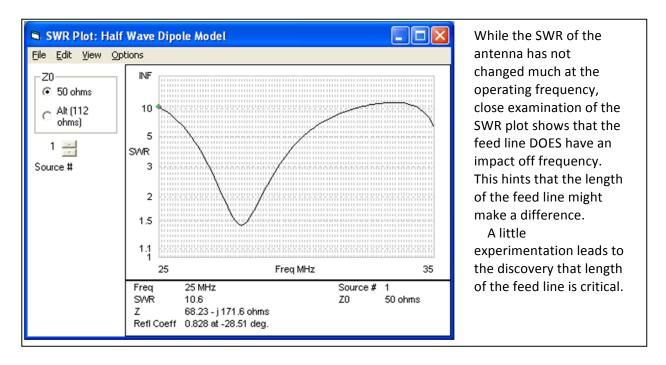
The next experiment is to change the length of the feed line away from the 1 wavelength chosen. As it turns out, making the feed line .75 wavelengths will show a larger effect:
