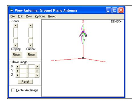
Feed line currents on elevated ground plane antenna. Perfect choke is used at the feed point. Feed line is ½ wavelength long and therefore resonant. This is the worst case.
