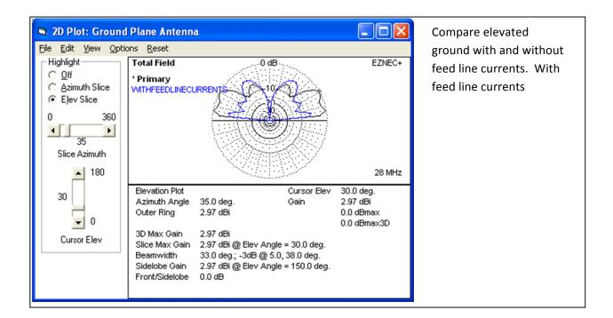
To drive home the point of this section, consider the original half wave dipole center driven. Below that one places a second, half wave vertical dipole. The two dipoles are NOT connected. Notice the currents and the gain pattern. From these two graphs it is easily seen that significant feed line currents can be induced and have a significant impact on antenna performance EVEN when not physically connected. One simply must take induced currents into account when deploying an antenna.
