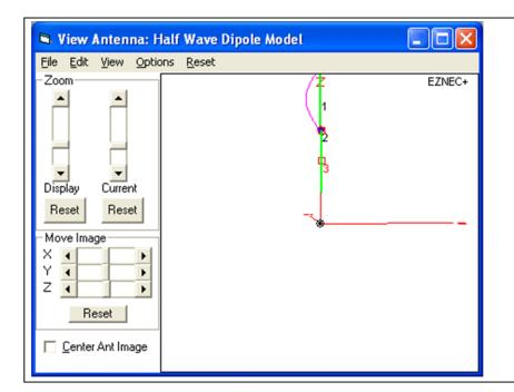
A second choke is placed at the high current path on the feed line. Feed line currents are now eliminated.
