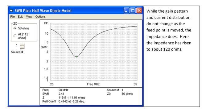
Next we drive the antenna from the 3% point. Again, the current distribution and gain patterns do not change and so are not shown. And again, the feed point impedance changes significantly:
