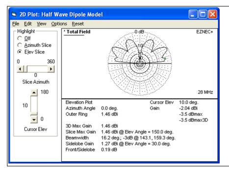
Indeed, introducing this second choke has changed the gain pattern. A great deal of RF energy is being launched upward.
