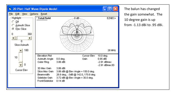
Still, there is significant current flowing in the feed line. This not only affects the performance of the antenna but also can affect safety.
