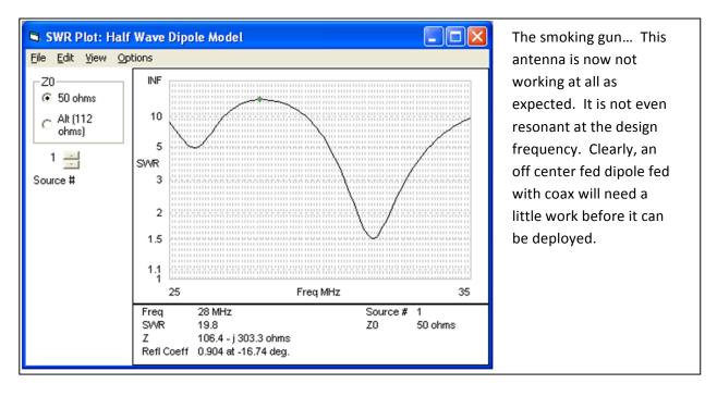
Thus, running the feed line at 90 degrees from the feed point is not sufficient to eliminate feed line currents. A few other cases are now examined.
