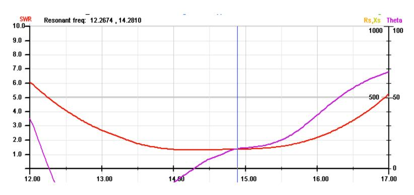
SWR Less than 2/1 from 13.75 to 15.75 MHz.
