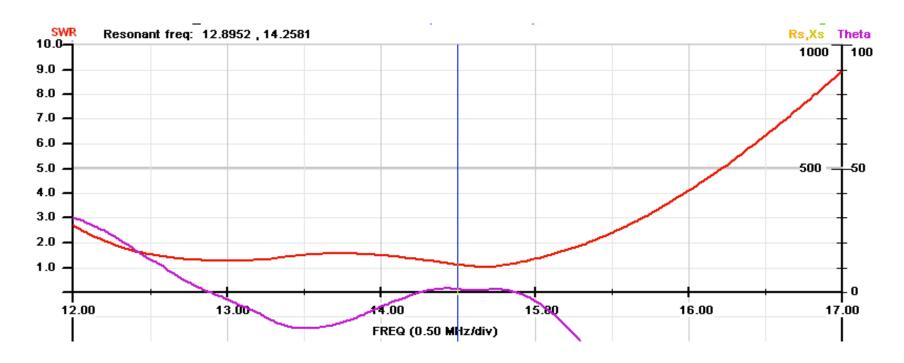
SWR Less than 2/1 from 12.5 to 15.5 MHz.
